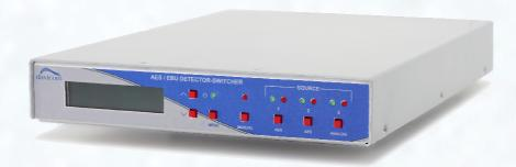
The Davicom DADS-01 is a digital audio detector and switcher. This device has the capability of sensing errors and silences in the digital audio input stream and automatically switching to a second AES signal, or to a third analog source. Besides operating automatically, the DADS-01 can also be operated manually, either locally or remotely, through its rear panel parallel I/Os or through a USB connection.
