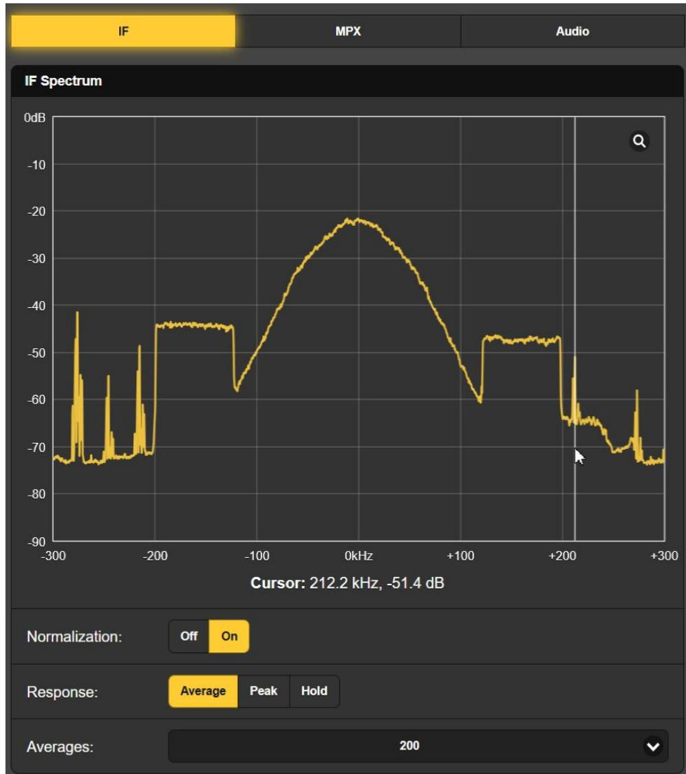
Clicking the magnifying glass in the corner will toggle to a full-screen display, and mousing over the display area brings up the cursor (white arrow vertical line) shown. The exact frequency and level at that point is presented below the spectrum.
