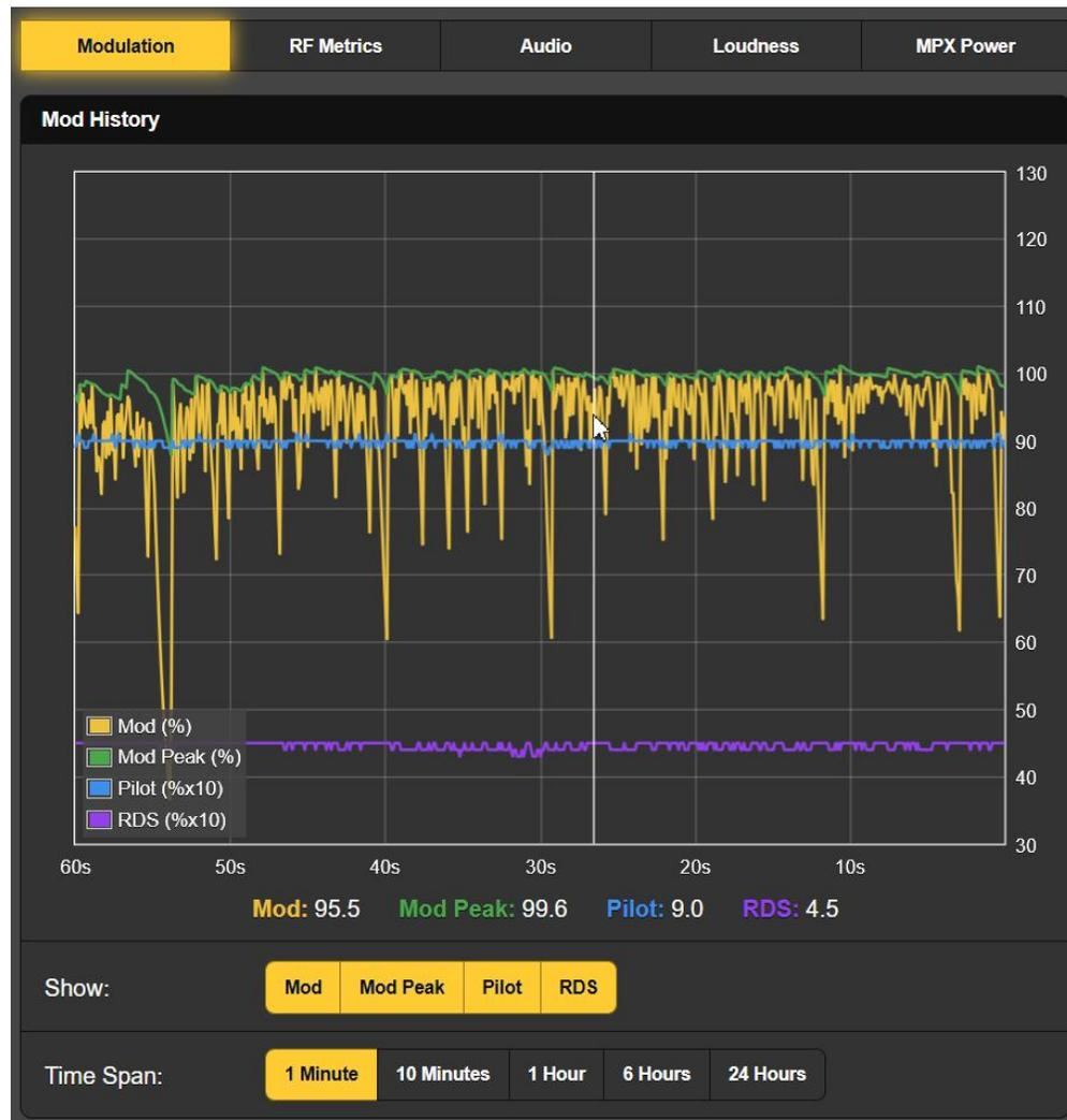
Note the Show: buttons below the screen. When all buttons are activated (by default as pictured), all four parameters are displayed above in different colors. If a particular display is confusing, you can easily turn-off those measurements you don't need to see.
