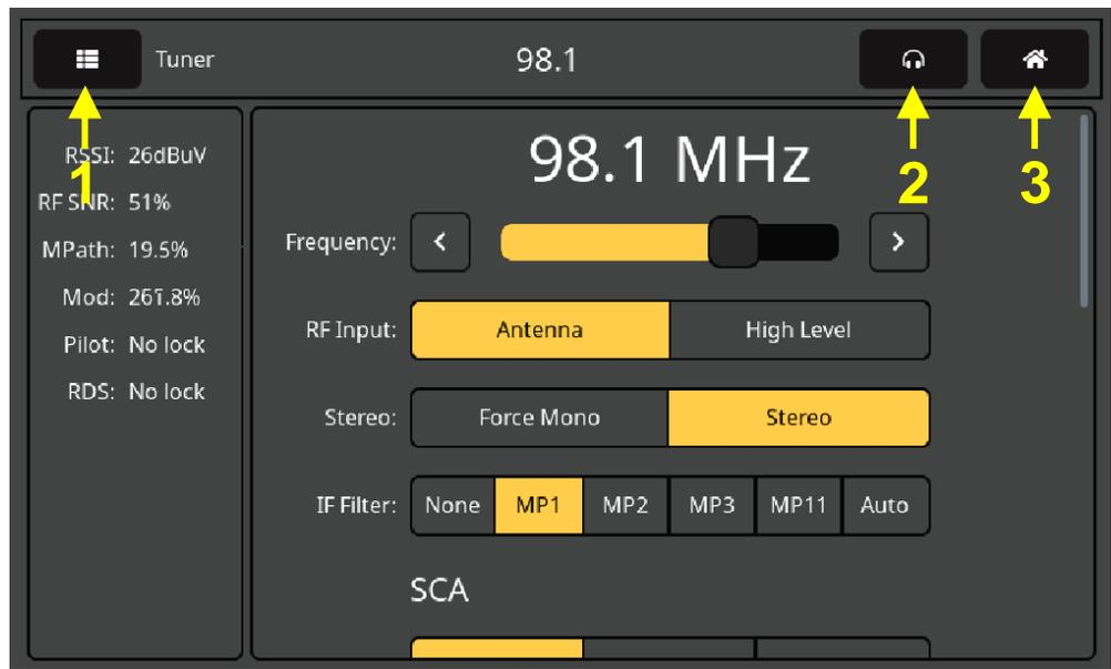
Arrows in the illustration identify items in the LCD screen header. An additional icon will pop up in the header when an alarm is triggered, just to the left of the headphone symbol. Touch that icon to show the alarm panel screen.
