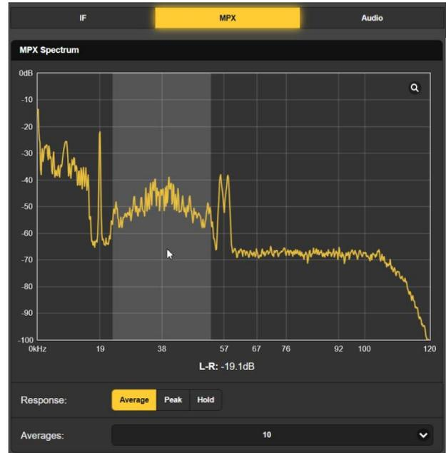
Set Response: to Average for a stable and meaningful display, the default 10 FFT Averages: is a good compromise for a dynamic, yet easy-to-read plot. Selecting Peak will reveal peak levels of the spectrum components, and Hold accumulates the highest peak value for as long as it remains selected.
