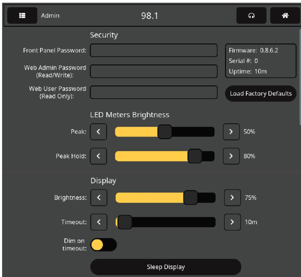
The Admin menu hosts Security settings. In addition it displays the unit's current firmware version and serial number, and shows how long the 541 has been running since AC mains power was last applied. Housekeeping features that show up here, along with a few more that can be accessed only through the Webpages interface, will be detailed later in this manual. This LCD-touchscreen Admin menu also gives the only access to front-panel display brightness and timeout options.
