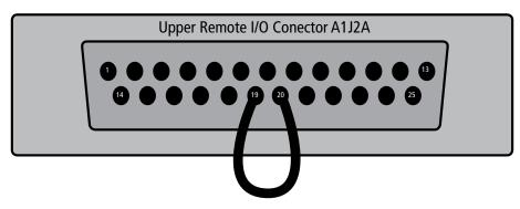
Install the interlock jumper (Part # 211-5060) between pins 19 and 20 of the REMOTE I/O-A (A1J2A) connector.
