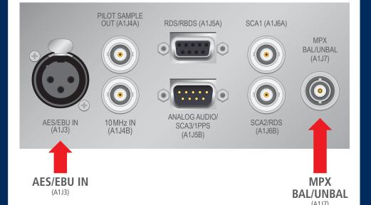
Default MPX input configuration is balanced (BAL). Refer to pre-installation manual to configure for unbalanced (UNBAL).
