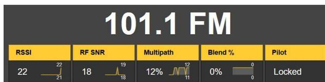
With the exception of Pilot, which indicates only a Locked or an Unlocked condition, each of the other four quality notations is accompanied by a scrolling 30-second graphical history, plus low and high values over the same period.
