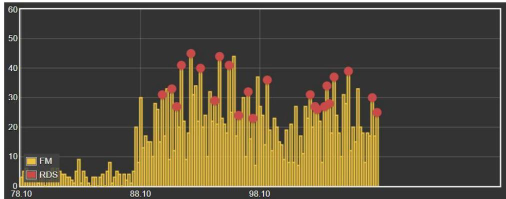
FM carriers are displayed as vertical bars, the height indicating the relative signal strength in dBuV per the annotation to the left of the plot. Had this scan been done in the simple RSSI: mode, all stations would show up just as yellow bars.
