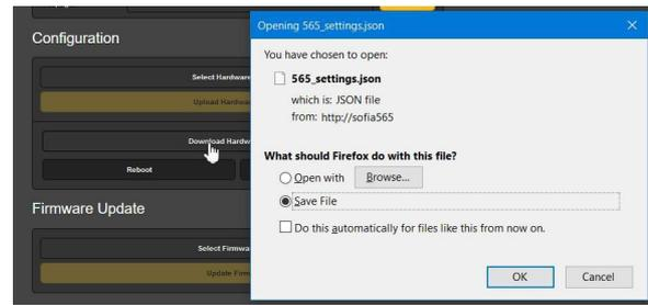
To upload (restore) a saved setting, first click Select Hardware Profile..., navigate to the folder where the profile has been saved and, when prompted, Open the file. Then click Upload Hardware Profile. This will replace all set-up parameters currently loaded and running in your SOFIA 565 with the saved ones.
