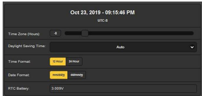
(Hours): slider for the proper offset from Universal Coordinated Time for your area. In this example, the -8 represents West Coast US (Pacific) time. The time at the top of the page will update immediately, so you can simply drag the slider until the time shown here agrees with that big clock on the wall.
