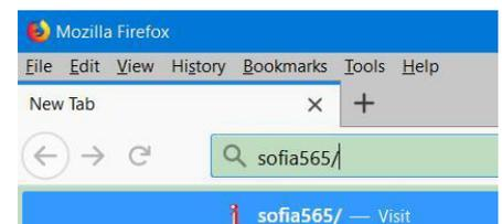
here. The entry is not case-sensitive in this instance. Non-Windows browsers may require you to enter the complete IP address of the unit, which you can always find by front-panel navigation to Setup / Network / IP Settings.
