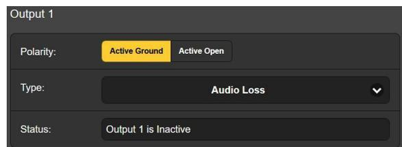
It could as easily have been set to deliver ground on that terminal all the time, and then go **Active Open** (ungrounded) when the alarm is received.
