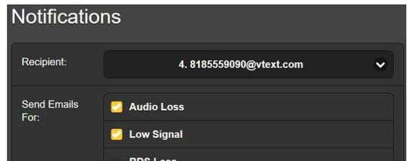
In this abbreviated example, the Chief Engineer will receive a text message on his phone for Audio Loss and Low Signal alarms. When you've finished with this Recipient, proceed to the next. A Save command is not necessary in this operation.
