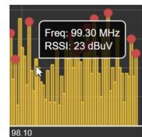
A yellow bar with a red dot indicates that the station carries RDS information. (The red dot shows only when the Scan Type: is set to RSSI + RDS.) Hovering over the red dot will show Freq: and RSSI:, plus the RDS PI: code and Call: letters (in the US and Canada), and the PTY, or programming format of the station as shown in the second example on the right.
