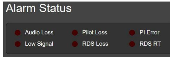
All six alarms give flashing notifications on the front-panel OLED screen, and are indicated in the Alarm Status area of this Web interface page as shown above. Any or all of the six are also able to initiate email or SMS/text messages to selected personnel, and alarms are logged for later analysis or finger-pointing.
