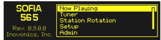
With the SOFIA 565 connected to your local network (LAN), use the jog wheel to navigate from the Main Menu to: Setup / Network / IP Settings.
