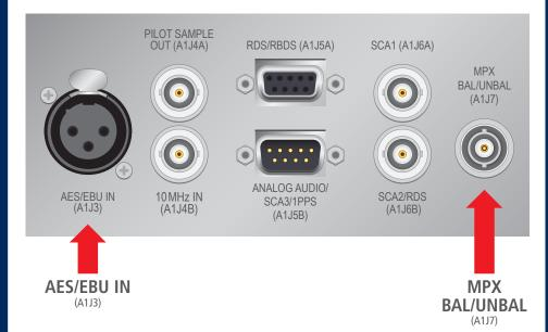
Default MPX input configuration is balanced (BAL). Refer to pre-installation manual to configure for unbalanced (UNBAL).
