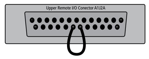
Install the interlock jumper (Part # 211-5060) between pins 19 and 20 of the REMOTE I/O-A (A1J2A) connector.
