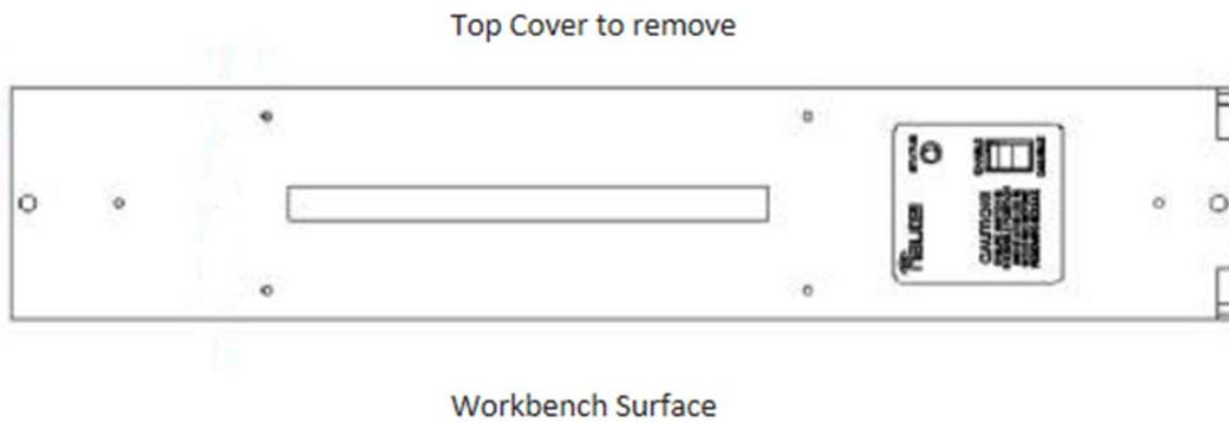
4. Remove the top cover (11 x M3 Phillips screws) and retain hardware.
