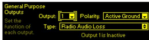
when the Radio Audio Loss is activated per the parameters set on Page 20. The other five, Output: 2 to Output: 5, may be assigned to other alarms (Type: Analog Audio Loss / Digital Audio Loss / Stream Audio Loss / Low Signal / RDS Error / Pilot Loss / HD Loss), and the alarm polarity set to Active Ground or Active Open.
