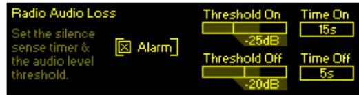
LOSS LED or the corresponding indicator on the Web interface Now Playing screen. Also there will be no closure at a rear-panel GPO terminal, nor will the AARON 655 send SMS/text or Email alerts to station personnel. Moreover, if failover to a secondary program feed depends on radio audio loss, that function will be inhibited as well. In short, the  Alarm box must be checked for any audio-loss (or other) alarm to activate.
