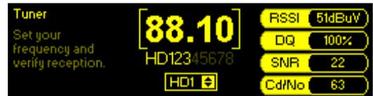
**NOTE:** When the AARON 655 is tuned to an HD Radio broadcast and the digital signal is lost, the receiver *does not revert* to analog-FM reception. The selection box at the bottom of the display sets the reception mode between FM and HD1 through HD8. This selection is ‘global’ and will determine the single off-air channel that will be received.
