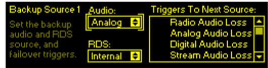
Whenever a higher-priority source returns and its alarm resets, the AARON 655 will automatically go back and reestablish that source as the on-air feed.
