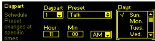
Once a programmed daypart begins it will continue indefinitely. Thus it is important to set up your 'normal' processing as a daypart as well, and program the scheduler to switch back when the alternative programming ends.
