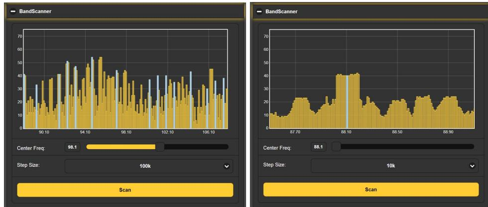
**NOTE:** The band-scanning function mutes the receiver audio during the scan cycle. Use this function only when off-air programming is *not* the source for the rebroadcast audio.
