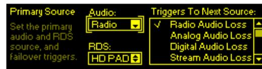
have selected Radio as the audio source (actually HD2 program audio in this case) and are reconfiguring HD PAD data from the HD2 broadcast into the RDS data format for rebroadcast. Here
