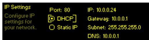
select:  DHCP to have your router automatically assign an IP address to the receiver. Once DHCP connection is established, the fields on the right-hand side of the screen will populate automatically.
